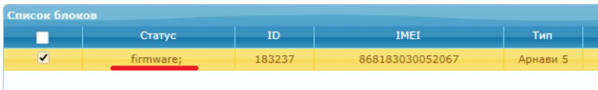
The screenshot shows the 'Status' column in the device list table highlighted with a red box. The entry for device ID 183237 now shows 'firmware;' instead of just 'firmware', indicating the new software has been assigned but not yet applied.
